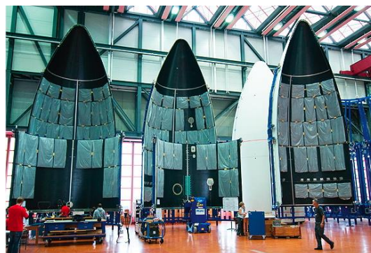
Final integration of RUAG Payload Fairings in Emmen, Switzerland. Photo: RUAG Space
